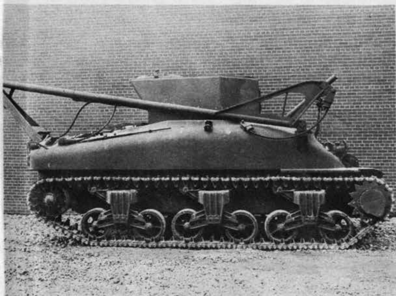
American tank-recovery vehicle has the hull and chassis of the medium tank and an armored crew compartment that resembles a tank turret. Loading crane with grapple hook is attached to rear.
